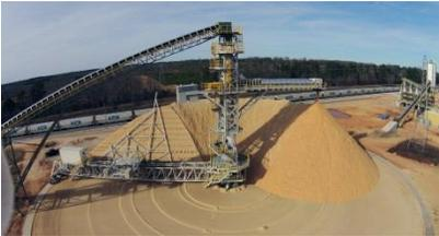
Figure 16 - Circular Blending Bed Stacker Reclaimer (Bruks Siwertell).
