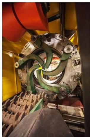
Figure 1 - A Ring debarker in the closed position.<sup>1</sup>
