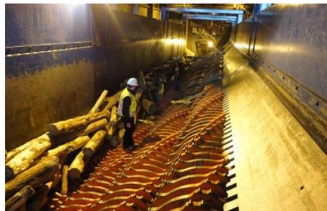
Figure 4 - Inside a High Capacity, End Discharge Rotary Debarker.
