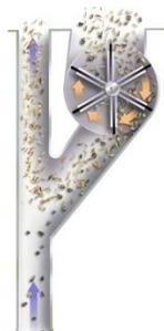
Figure 7- Air Density Separation System (<https://acrowood.com/specialty/air-density-separator/>).
