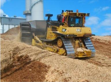
Figure 15 - Bulldozer pushing chips on a FILO chip storage pile.
