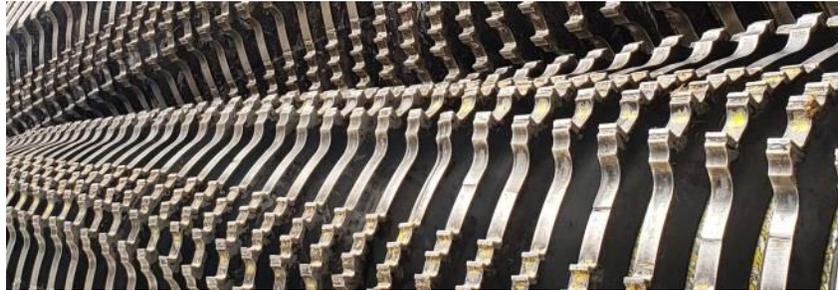
Figure 1 - Rotary Debarkers Rotors. The Abrader design and open bottom of the debarker are unique design parameters.
