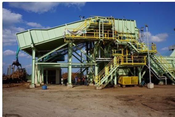
Figure 2 -Side Discharge Rotary Debarker
