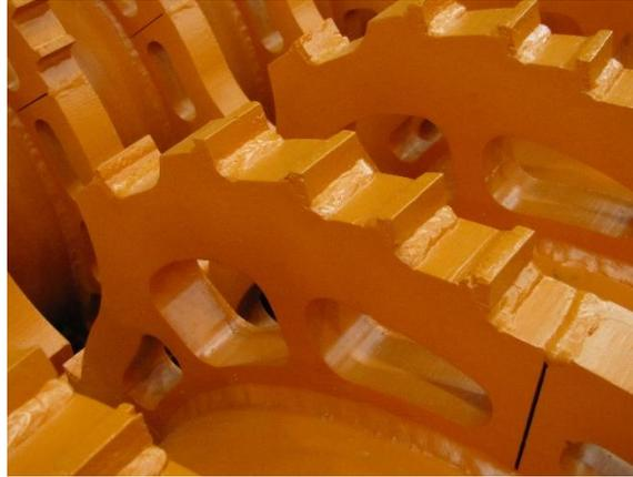
Figure 6 - Block-type Abrader Tips
