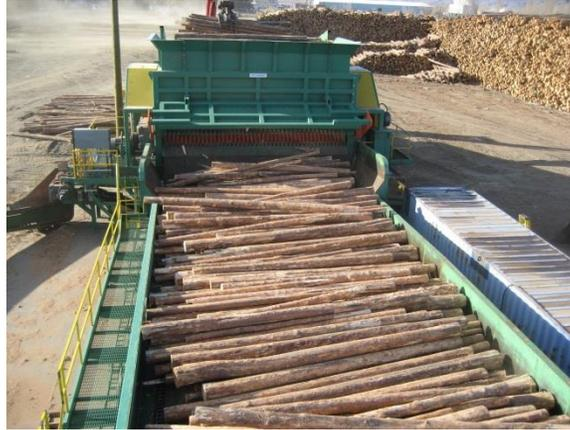
**Figure 7 - Debarked Logs on an Outfeed Deck.**
