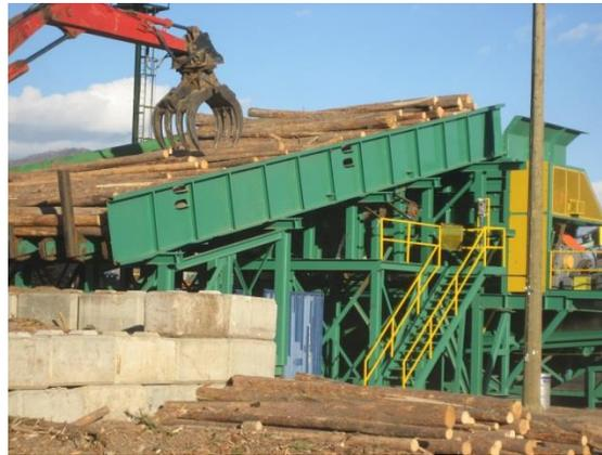
**Figure 5 - Infeed Deck to Side Discharge Unit Fully Loaded.**
