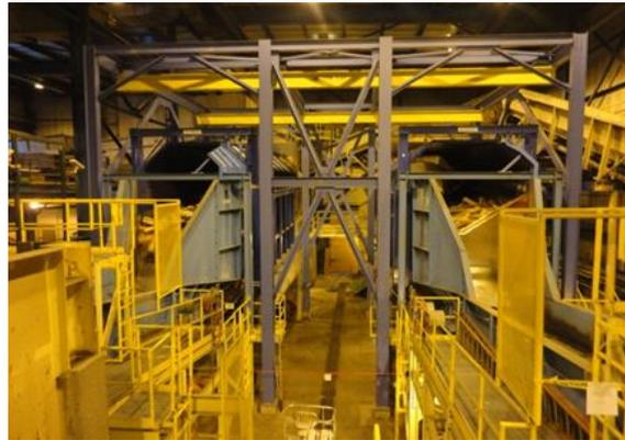
**Figure 3 - End Discharge Rotary Debarkers.**
