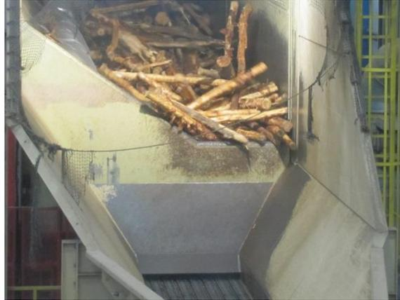
**Figure 4 - Gate Height on End Discharge Debarker is Critical for Debarker Efficiency.**
